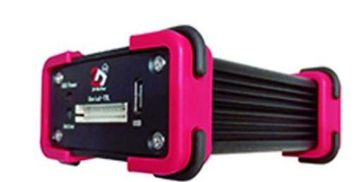
ZD-Shifter SU12 interconnects various devices using serial communication on RS232 standard. This innovative all-in-one level converter supports simultaneous bi-directional communication between USB, RS232 and UART interfaces with advantages of small size, low power consumption and high performance.
